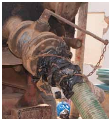
Figure 4.13 Example of an improperly maintained hose held together with plastic bags and twine (photo: David M. Robbins).
